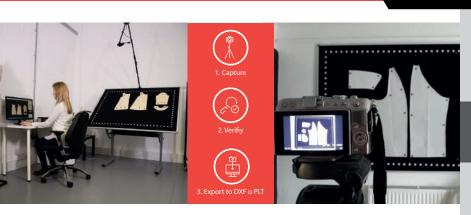
Our Velocity V-Shoot Digitizing Camera is an advanced solution designed to quickly and accurately transform physical patterns into digital files. Using high-quality photographic capture, this technology allows users to digitize patterns easily and efficiently, eliminating errors and streamlining workflow.
